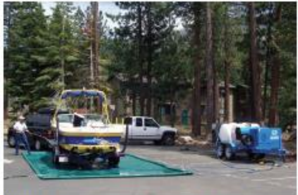
Wastewater collection pad used with portable decontamination unit (Hydroblaster)
